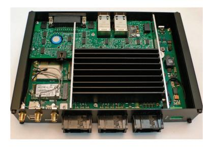
Weiß Elektronik & Software GmbH has developed a dedicated mezzanine card for analog inputs, TFT display support, GPS, acceleration and gyro sensors, and power outputs. It is mounted on the custom SBC. The WeMOTA G2 heatspreader couples directly to the housing and is milled out towards the module for an optimum fit.
