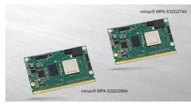
WeMOTA G2 is based on MicroSys miriac System-on-Modules with NXP S32G processors, which are predestined for use in vehicles thanks to native support of CAN, FlexRay and LIN, as well as TSN-enabled Ethernet and Ethernet T1. MicroSys currently offers two configurations, featuring either 4 Arm Cortex-A53 processors and 3 Arm Cortex-M7 processors, or 8 Arm Cortex-A53 processors and 4 Arm Cortex-M7 processors clustered as a dual lockstep pair.
