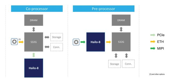
MicroSys also supports Hailo-8 Al accelerators on its NXP S32G platforms. Combining high computing performance with minimal power consumption, these accelerators are ideal for edge computing applications in vehicles.
