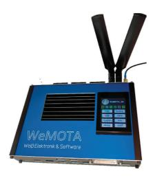
WeMOTA G2 from Weiß Elektronik & Software GmbH is a vehicle edge gateway that offers developers powerful edge logic for evaluating vehicle data in the field and for filtering out specific vehicle and environmental data that is relevant for their needs. This minimizes the amount of data to be transferred to the cloud. Over-the-air updates can be deployed at any time to reset the vehicle and environmental data parameters.
