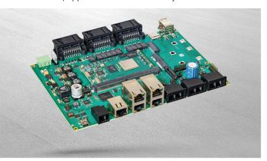
MicroSys' also designs custom specific carrier boards for its System-on-Modules. They are deployed as application-ready modular SBCs in the WeMOTA G2 system. Custom-specific designs can be implemented much more cost-effectively on such carrier boards than with a full custom design.
